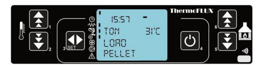
After ignition of pellet, and after tempereture of flue gasses raise on value of 50°C, regulation receives signal that fire is on and boiler continues to work with set values.
