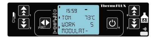
If temperature rises above set temperature by 2°C, boiler will be shut down automatically and on display will be written **WAIT COOLING**.
