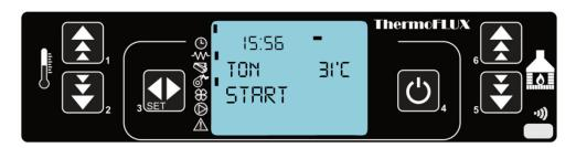
**START** will be displayed, on the left side of display we see that igniter and suction fan are activated. Mark **tON** is showing that room thermostat is connected or overbridged on connection for room thermostat (deafult). After that, on display we have text **LOAD PELLET** and on the left side we see that feeding of pellet is activ.
