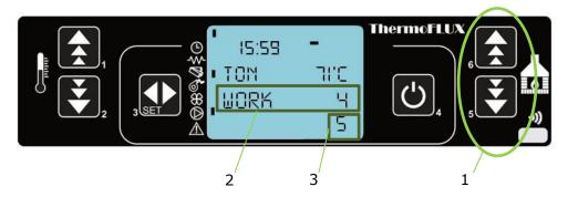
Regulation on the boiler is set in the way to modulate (power goes into lowest one) it's work when 4 C is reched below set temperature – **read 6.5 Modulation.**
